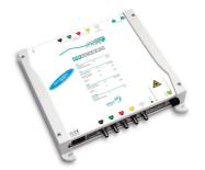
Innovative solution that allows you to transmit the entire TV band, including radio signals, and an entire orbital position on a single fibre. Optical transmitter suitable for CWDM (Coarse Wavelength Division Multiplexing) technology for the distribution of up to 4 orbital positions on a single fibre. Wavelength 1510nm, DFB at 7dBm (dimensions 230x230x50mm)
